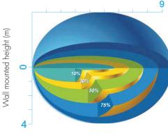
Ceiling mounted detection pattern (m)
